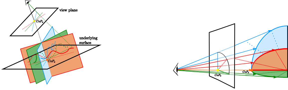
Figure 3: The left diagram shows that the coherent visible curves for an underlying plane are a pencil of lines on both the surface and the view plane, intersecting respectively at CoP_s and CoP_v . The right diagram shows that the coherent visible curves for an underlying sphere are the set of great circles intersecting at the CoP_s for the surface, which maps to a pencil of lines on the view plane meeting at the CoP_v .
