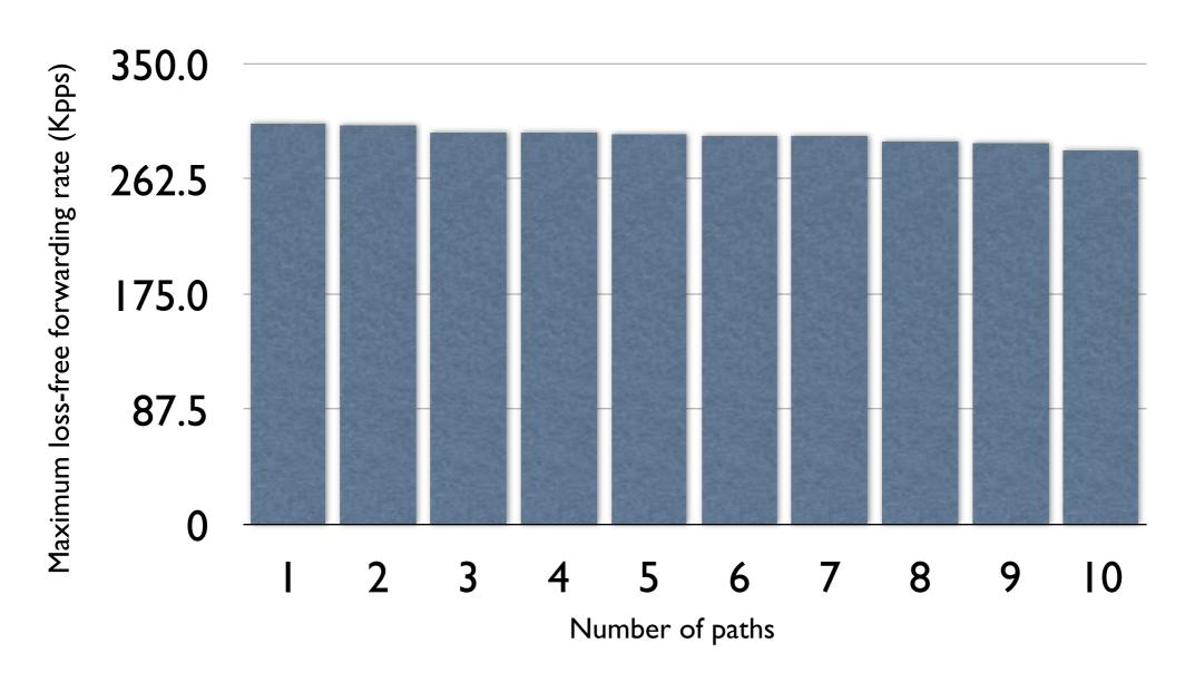
NetPath enables more efficient use of resources. Slight performance degradation is due to scheduling overhead.
