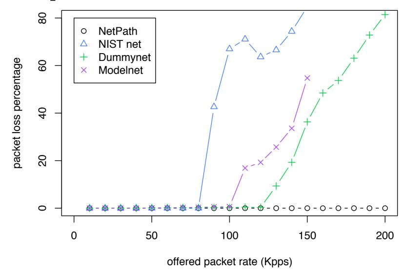
NetPath accurately emulates delay without introducing packet loss for much higher rates than other emulators.
