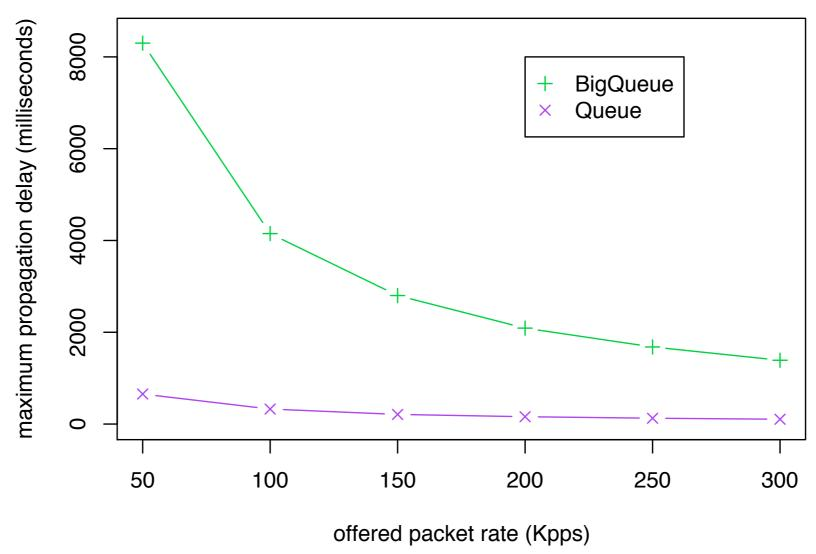
Using available system RAM enables longer delays at higher packet rates.
