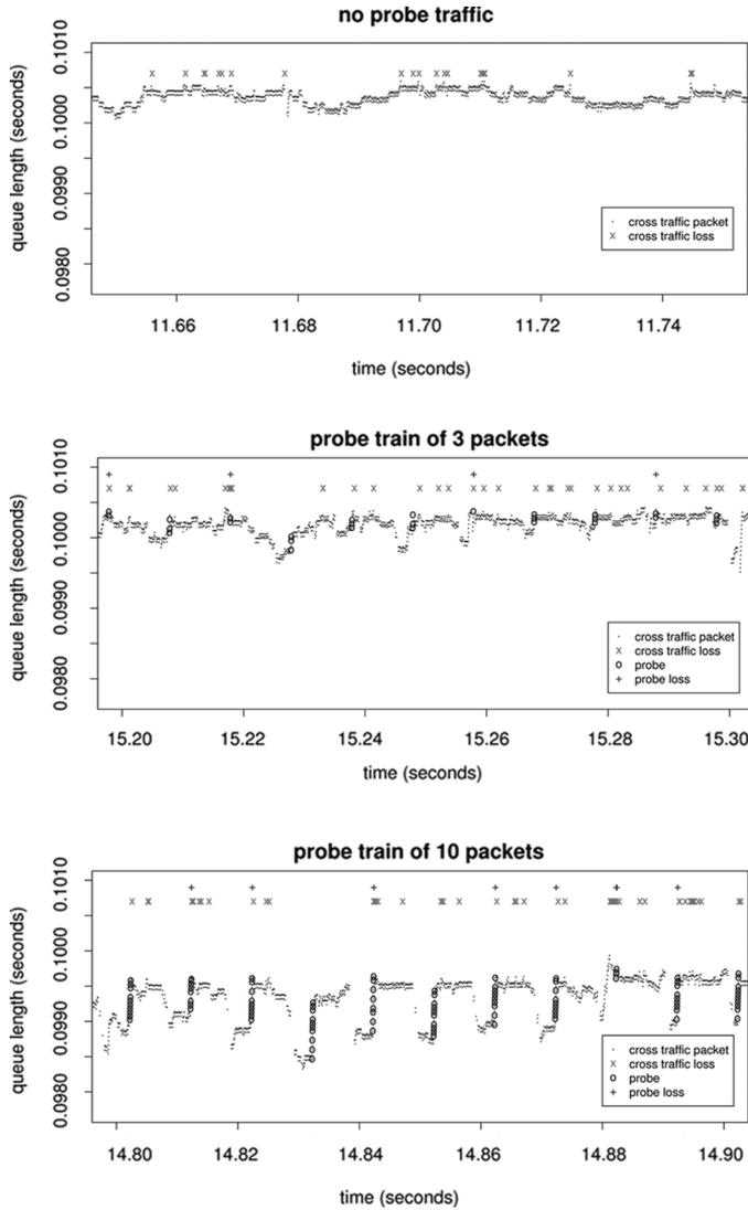
Fig. 5. Queue length during a portion of a loss episode for different size loss probes. The top plot shows infinite source TCP traffic with no loss probes. The middle plot shows infinite source TCP traffic with loss probes of three packets, and the bottom plots shows loss probes of 10 packets. Each plot is annotated with TCP packet loss events and probe packet loss events.
