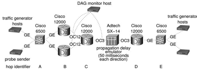
Fig. 2. Laboratory testbed. Cross traffic scenarios consisted of constant bit-rate traffic, long-lived TCP flows, and web-like bursty traffic. Cross traffic flowed across one of two routers at hop B, while probe traffic flowed through the other. Optical splitters connected Endace DAG 3.5 and 3.8 passive packet capture cards to the testbed between hops B and C, and hops C and D. Probe traffic flowed from left to right and the loss episodes occurred at hop C.
