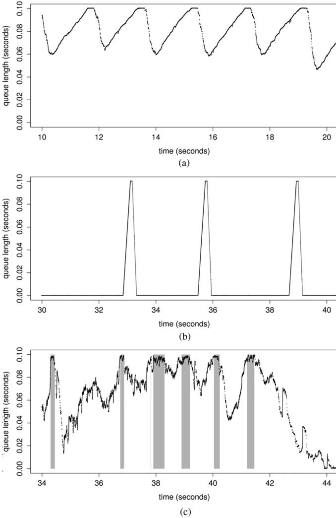
Fig. 3. Queue length time series plots for three different background traffic scenarios. (a) Queue length time series for a portion of the experiment with 40 infinite TCP sources. (b) Queue length time series for a portion of the experiment with randomly spaced, constant duration loss episodes. (c) Queue length time series for a portion of the experiment with Harpoon web-like traffic. Time segments in gray indicate loss episodes.
